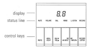
Although there are many sophisticated features, all commonly used functions require only one key press. To access the less commonly used functions, such as balance, two keys must be pressed at the same time. The status of the WAKONDA is always indicated through the row of indicator lights.
